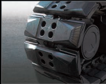
BS Geo Grip, bolt on rubber inserts
