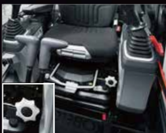
Adjustable Height Joystick Consoles
