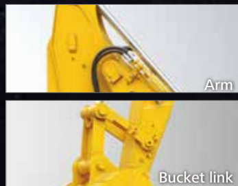
Machine Guidance Ready Brackets
