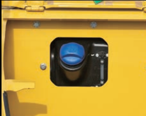
DEF Tank The DEF fill is located inside the locking tool box.
