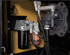
Engine Oil Filter / Pre-Filter with Integrated Water Separator
