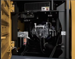
Right Side (Ground Level Maintenance) Hydraulic pump and engine filter compartment.
