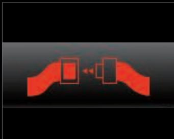
Seatbelt Unfastened Indicator on Monitor
