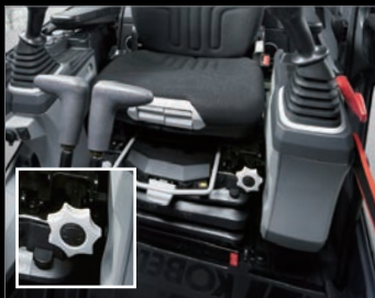
Adjustable Height Joystick Consoles
