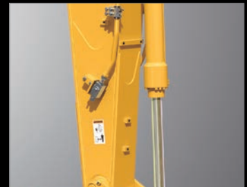
Quick Coupler Piping Brackets
