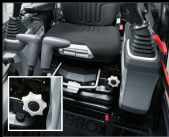
Adjustable height pilot valves
