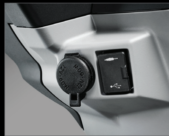
USB charging port / 12 V power socket
