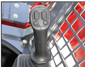
Pilot Operated Controls
