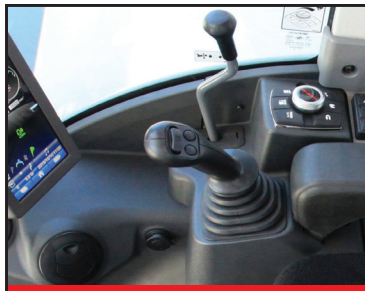
Hydraulic Pilot Controls
