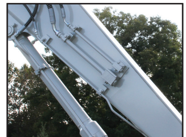
Auxiliary Hydraulic Lines
